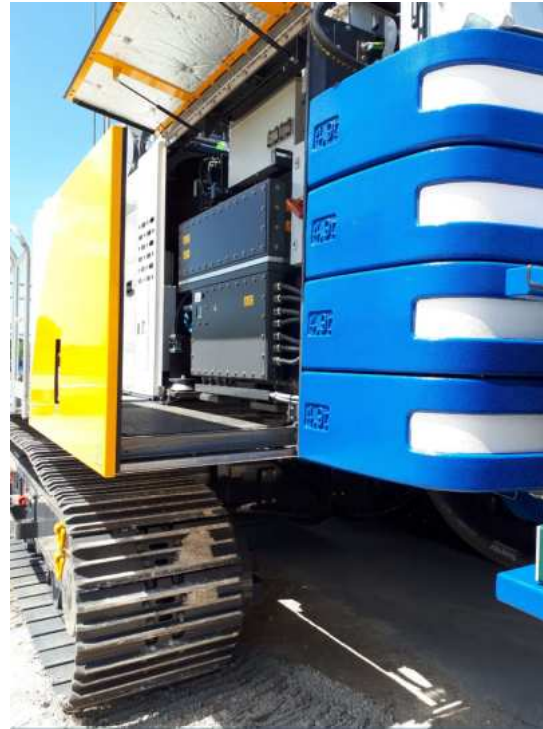
405kW electric motor unit
